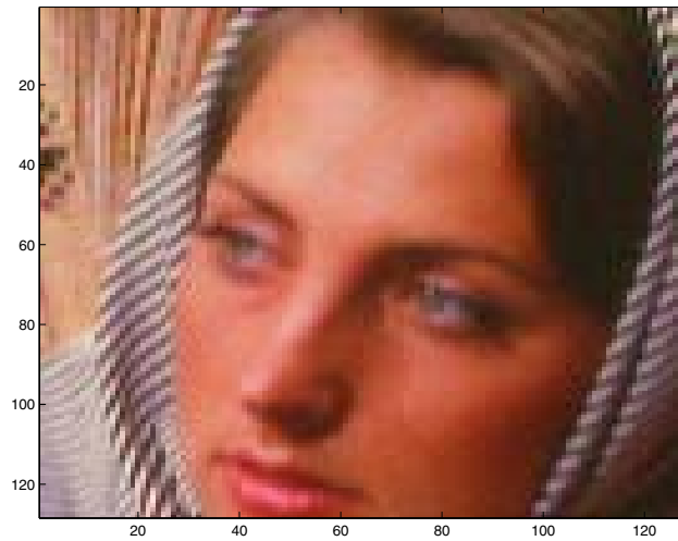
FIG. 5.3. The image recovered by the least squares method. The observed image is used to calculate \beta . PSNR = 27.79db.
