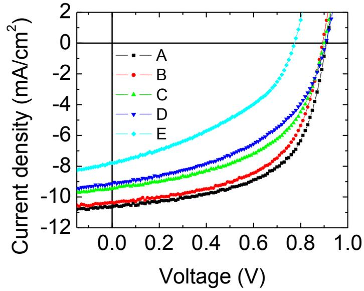
Figure 3. OPV cell performance of PCDTBT samples A to E with a structure of ITO/MoO<sub>3</sub>/PCDTBT:PC<sub>71</sub>BM/LiF/Al.
