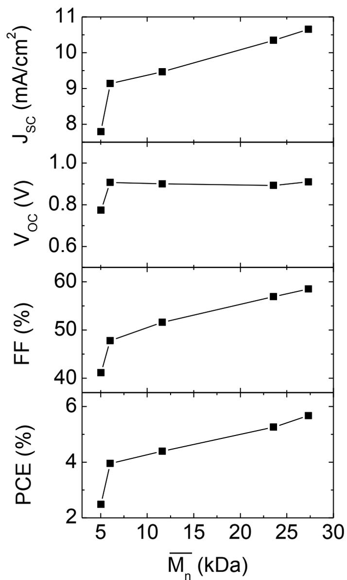
Figure 4. OPV cell parameters,  $J_{SC}$ ,  $V_{OC}$ ,  $FF$ , and,  $PCE$  vs the overall average molecular weight,  $\overline{M}_n$ .  $J_{SC}$  and  $FF$  have strong correlations with  $\overline{M}_n$  resulting in higher  $PCE$  with higher  $\overline{M}_n$ .
