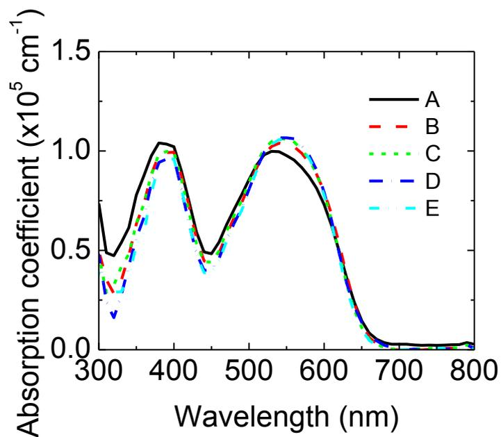
Figure 5. Absorption coefficients of PCDTBT A to E.
