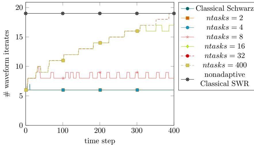
FIG. 7. WRAP for advection-diffusion equation with  $\nu = 0.005$ : plot shows the number of waveform iterates at each time step required to reach the same final tolerance for varying numbers of simultaneous tasks.
