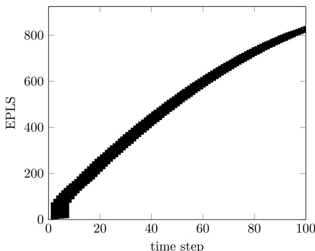
FIG. 6. Classical Schwarz coupling conditions: bars denote computation of the waveform iterates for each time step ( $x$ -axis) relative to when they are computed in the simulation ( $y$ -axis) for the case  $ntasks = 8$ . Here, the wall time unit is the amount of time it would take to compute one parallel solve. This WRAP method using  $ntasks = 8$  requires 841 EPLS.
