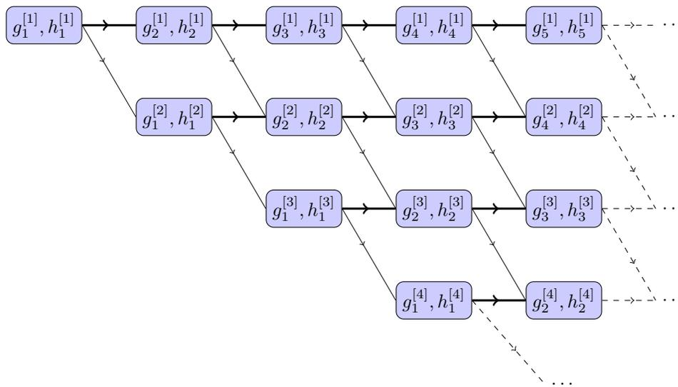
FIG. 1. *Dependency graph for SWR. The variables within the purple boxes denote the outputs of the `integrate` routine. The width of the arrows reflects the amount of information that needs to be passed to the newly spawned tasks. If the execution of each task (purple box) takes roughly the same wall time, each column of tasks can be simultaneously computed if sufficient processors are available.*
