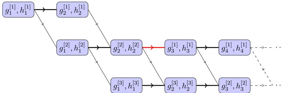
FIG. 3. Dependency graph for SWR if two iterations are performed in  $I_2$  before we begin iterating in  $I_3$ , i.e.,  $g_2^{[2]}$  is used instead of  $g_2^{[1]}$  to compute  $g_3^{[1]}$ . Each column has only two tasks, i.e., only two time-parallel tasks can be simultaneously computed ( $ntasks = 2$ ).
