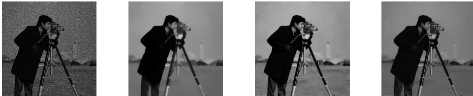
Fig. 11. The observed image corrupted by Gaussian noise (subfigure 1). The result of AA model (subfigure 2) using \alpha = 0.07 , the result of CONVEX model (subfigure 3) using \alpha_2 = 8 \times 10^{-4} , the result of our model (subfigure 4) using \alpha = 1 \times 10^{-4} .
