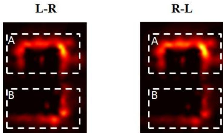
Fig. S3 The zoom-in view of the near field distribution from a single petal.
