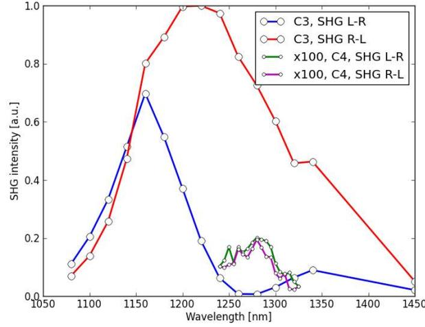
**Figure S1: Comparison of SHG spectra between Trisceli- and Gammadion- type plasmonic nanostructures.** The pumping power for C3 and C4 nanostructures are 20 mW and 60 mW, respectively. The intensity of SHG from Gammadion-type nanostructure is magnified by 100 times. The measured SHG spectra have opposite circular polarizations (L-R and R-L) as that of the normally incident illuminating light, where the abbreviation of L and R represents for LCP and RCP, respectively.
