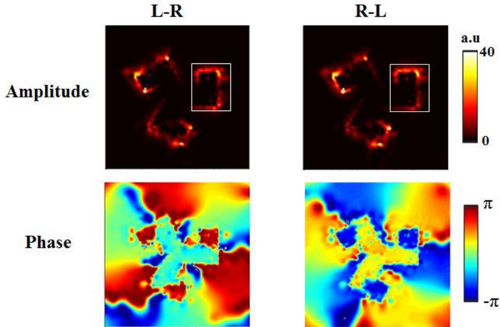
**Figure S2. Amplitude and Phase distribution** on the bottom surface of  $\overline{f_r} \cdot \overline{P_L}$  and  $\overline{f_L} \cdot \overline{P_R}$  (local field contribution to far-field) for left and right circular polarizations at 1291 nm. The first row shows the amplitude distribution while the second row represents the phase distribution.
