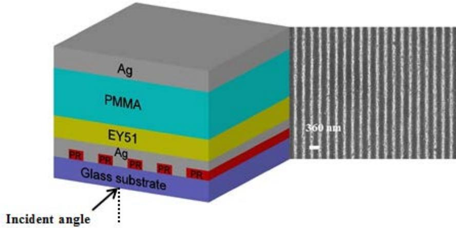
Figure 1. The hybrid plasmonic microcavity configuration and the SEM image of grating surface quality.
