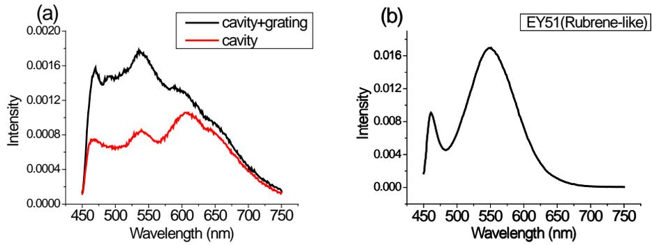
Figure 3. The PL emission from (a) the plasmonic and photonic microcavity, (b) EY51 thin film.
