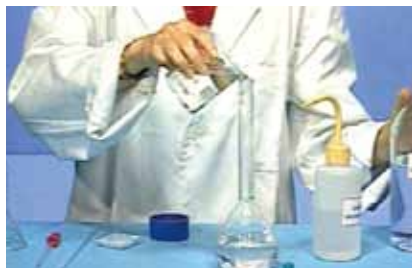
Picture 2 - Transfer the NaOH solution into a 250 mL volumetric flask.
