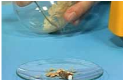
Picture 5 - Collection of crude caffeine after simple distillation.
